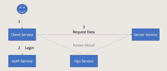
While the user login to an application is facilitated by the Symbio Authorization Service (Auth Service), the communication among services is secured by the Ops Service. This is especially true for services providing access to confidential data (in contrast of processing only provided data):
